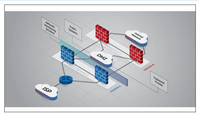
Figure 1: Network perimeter with firewalls and a DMZ
